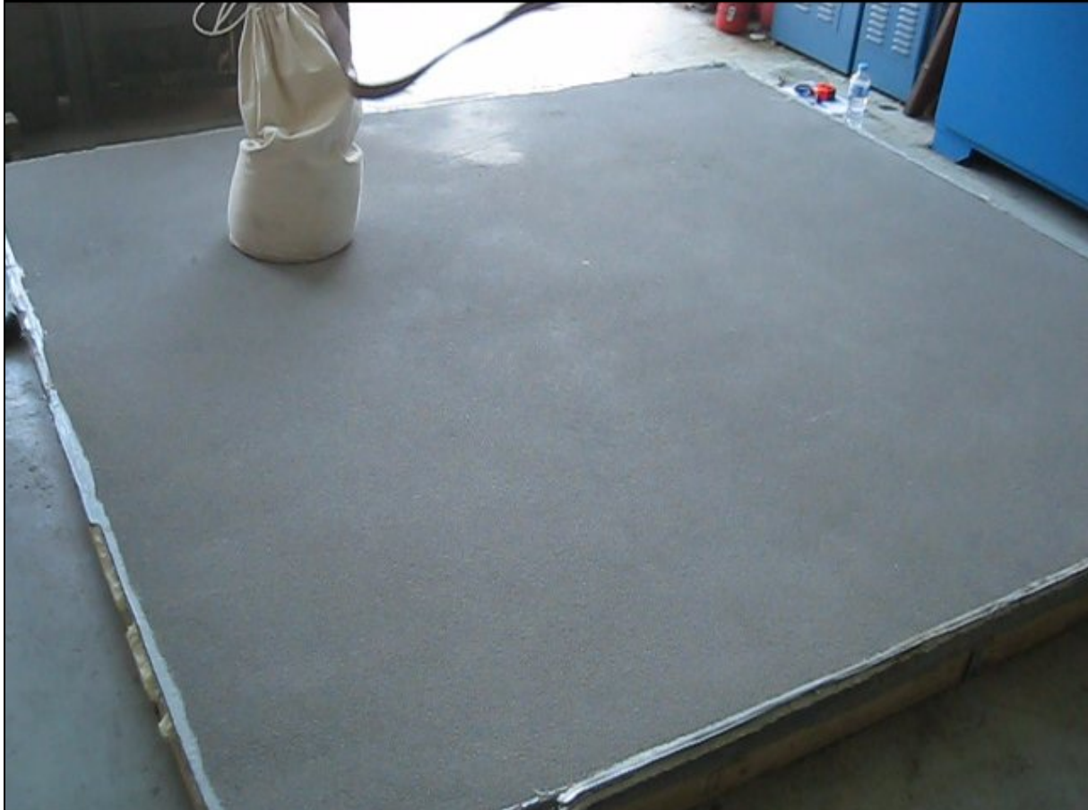
Figure 3: Sandbag impacting at Point 1
