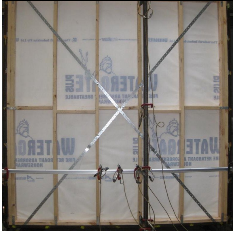
Figure 6: Serviceability deflection setup
