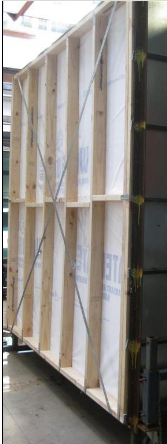
Figure 8: Test specimen under ULS negative pressure
